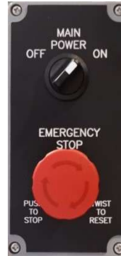
MASTER POWER / E-STOP
